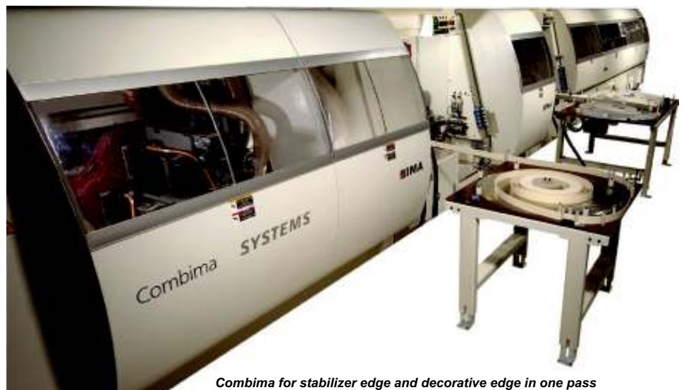
Combima for stabilizer edge and decorative edge in one pass
