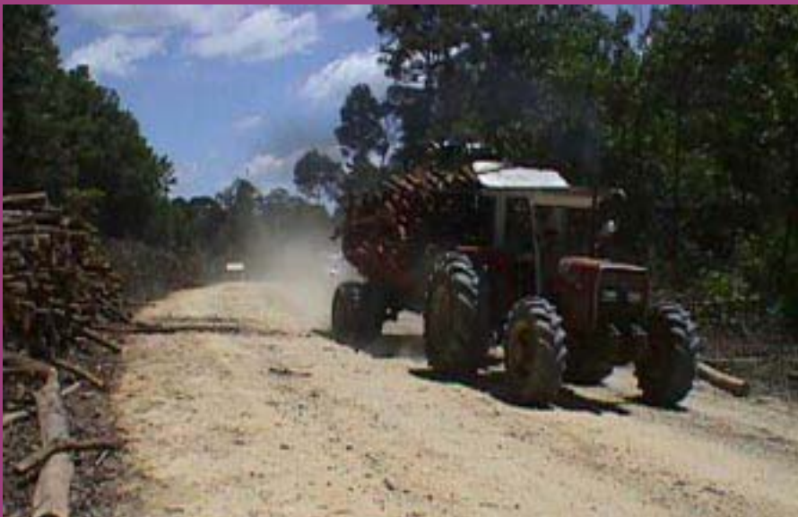
Unlike traditional forwarders, wheel tractor coupled forest trailers can do 40 km/h on roads, making it unnecessary to reload the logs to trucks for short distances.
