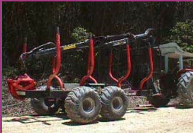
Nokka trailers were lengthened by 3 feet and fitted with an extra pair of side poles to accommodate two tiers of short logs.
