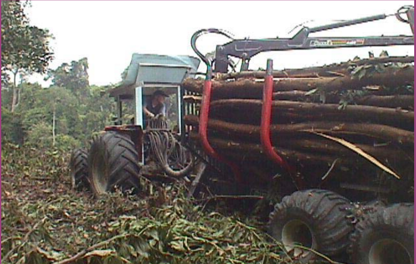
Here, Nokka 12 ton forest trailer is coupled to an old MF-390 wheel tractor whose roof has been tilted up to give better view to the loader which operated by the excavator type levers.
