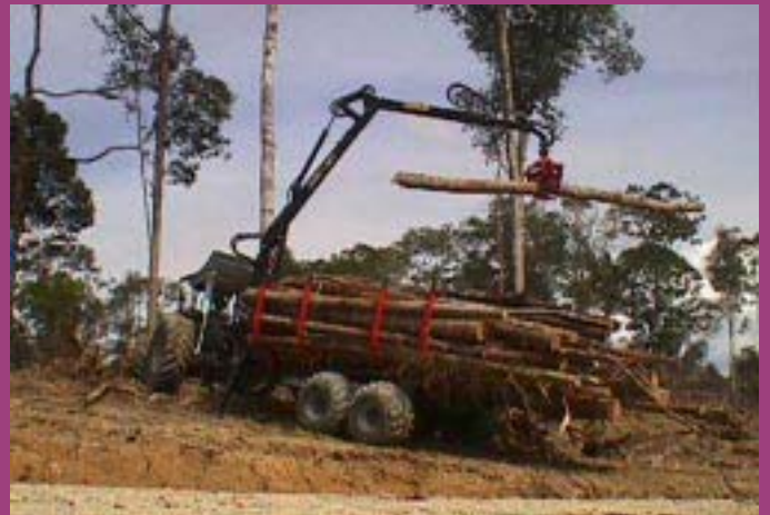
Nokka can take full 12 tons of logs whether they are short or long. Designed primarily for plantations, the trailer is here loading mixed tropical logs in Sumatra.
