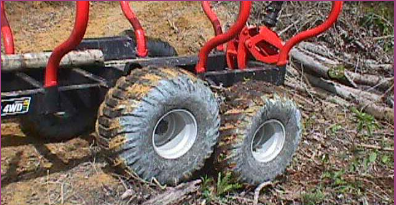
The wheel tractor PTO pump operates a 4-WD system to the rear low ground pressure balloon tires. The system is activated from the cabin and deactivates automatically when speed exceeds set limits.
